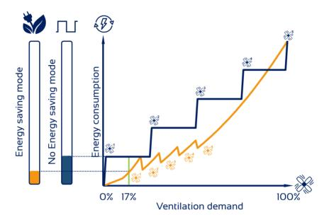
The energy mode is designed to optimize your fan performance and energy efficiency. It will progressively start more and more fans at the lowest possible speed, and then, once they are all on, the module will gradually increase fan speed for all of them as the ventilation demand increases.
